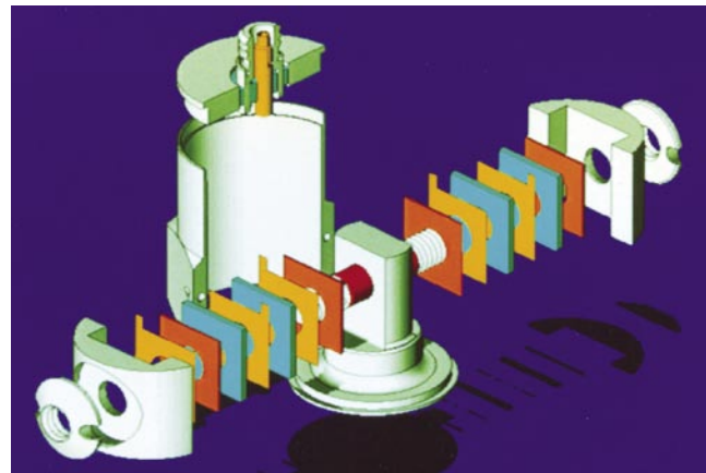
Figure 7-17 Shear piezoelectric accelerometer (courtesy Endevco, Patrick L. Walter, S/V 6/99)
