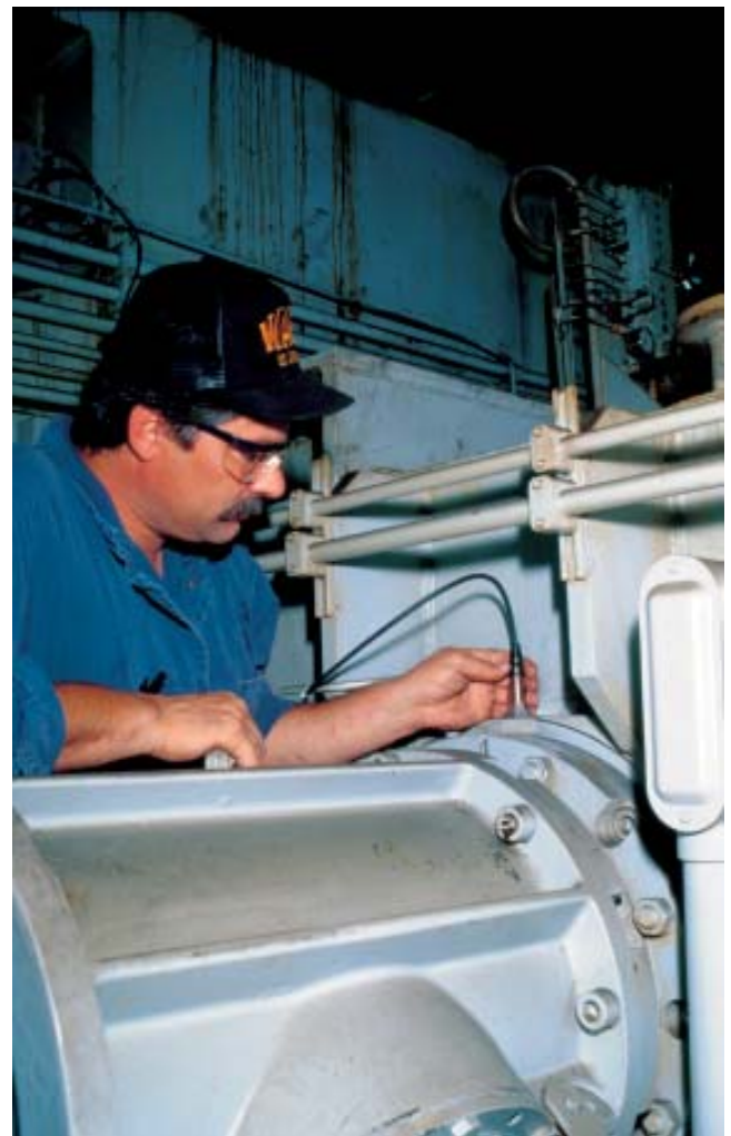
Figure 1-20 Measuring a machine's vibration
