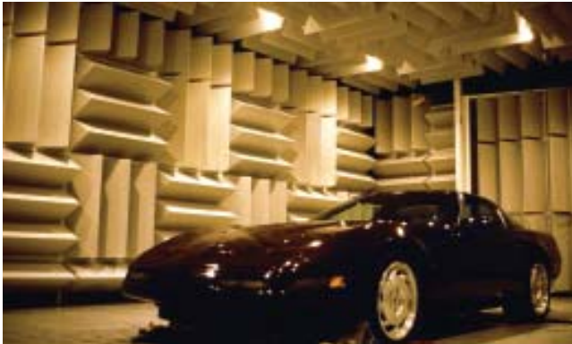
Figure 1-29 Noise test in hemi anechoic room
