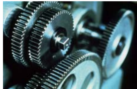
Figure 1-12 Gear train as vibration source
